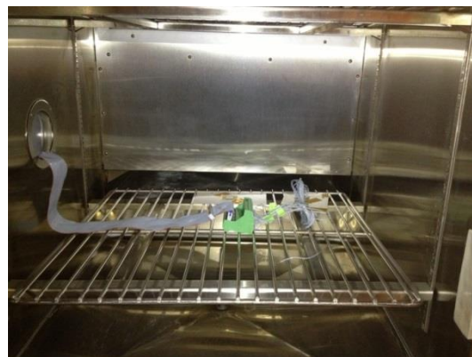
Figure 9-20: Test specimens within thermal cycle chamber
